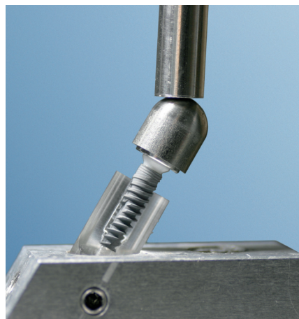
Figure 2: 30° Off-axis Fatigue Testing
